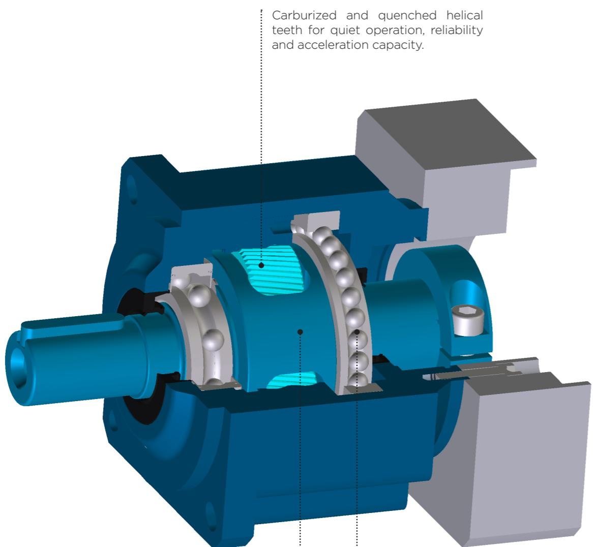
The caged planet carrier provides stiffness, reliability and acceleration capacity to the gearbox.
