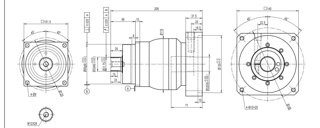
Note 1: This drawing shows the dimensions of X-Treme-SQ-ST-100 - 1 STAGE (this drawing is common to ratios 3 to 10)
