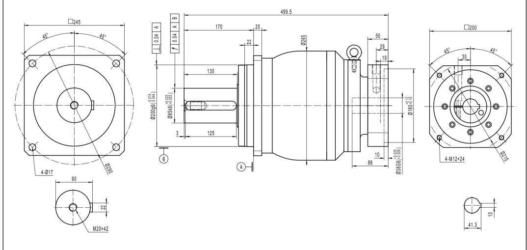
Note 1: This drawing shows the dimensions of X-Treme-SQ-ST-240 - 1 STAGE (this drawing is common to ratios 3 to 10)
