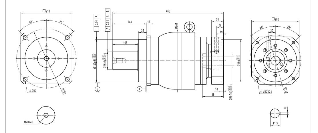
Note 1: This drawing shows the dimensions of X-Treme-SQ-ST-210 - 2 STAGES (this drawing is common to ratios 3 to 10)
