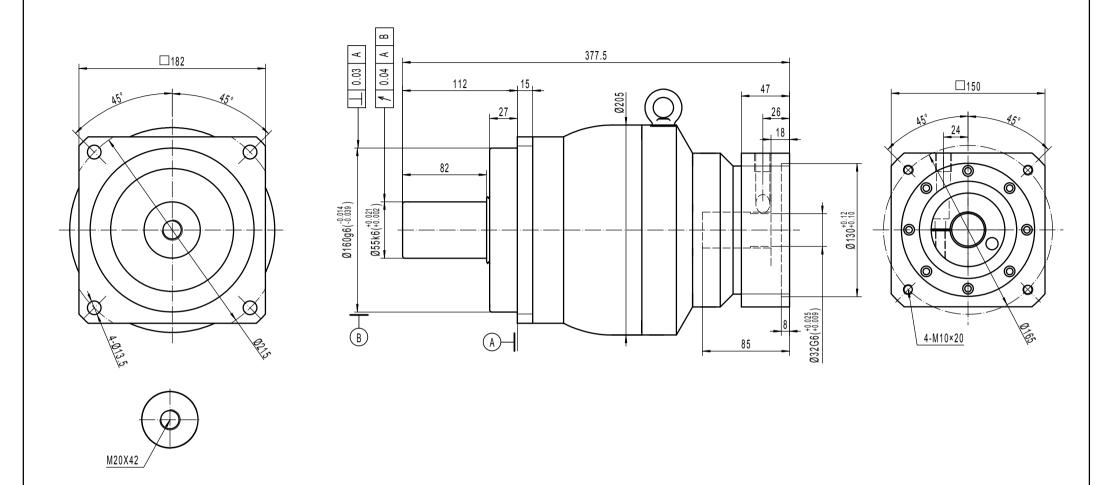
Note 1: This drawing shows the dimensions of X-Treme-SQ-ST-180 - 2 STAGES (this drawing is common to ratios 3 to 10)
