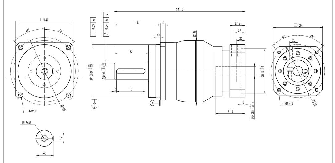
Note 1: This drawing shows the dimensions of X-Treme-SQ-ST-140 - 2 stages (It is common to all ratios from 12 to 100)
