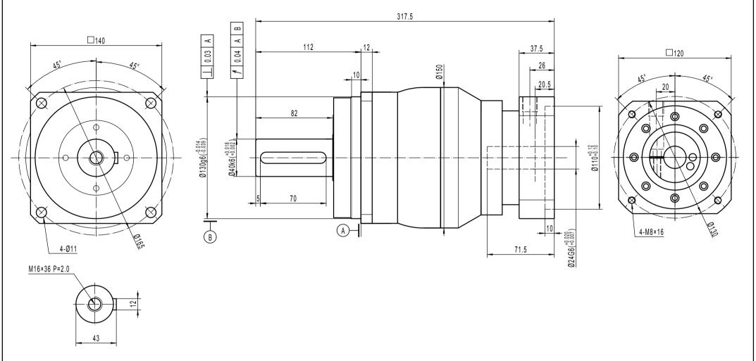
Note 1: This drawing shows the dimensions of X-Treme-SQ-ST-140 - 2 stages (It is common to all ratios from 12 to 100)
