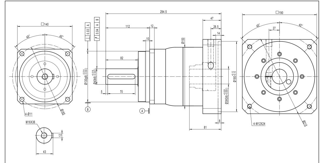
Note 1: This drawing shows the dimensions of X-Treme-SQ-ST-140 - 1 STAGE (this drawing is common to ratios 3 to 10)
