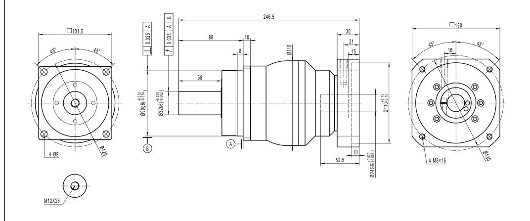
Note 1: This drawing shows the dimensions of X-Treme-SQ-ST-100 - 2 stages (It is common to all ratios from 12 to 100)
