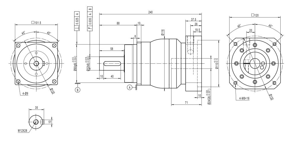
Note 1: This drawing shows the dimensions of X-Treme-SQ-ST-100 - 1 STAGE (this drawing is common to ratios 3 to 10)
