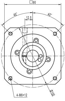
Note 1: This drawing shows the dimensions of X-Treme-SQ-ST-075 - 2 stages (It is common to all ratios from 12 to 100)
