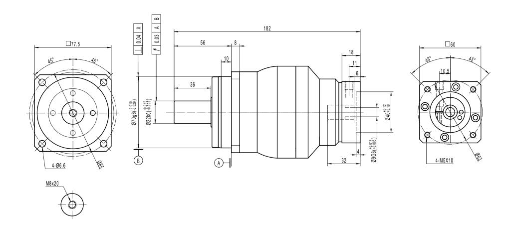
Note 1: This drawing shows the dimensions of X-Treme-SQ-ST-075 - 2 stages (It is common to all ratios from 12 to 100)
