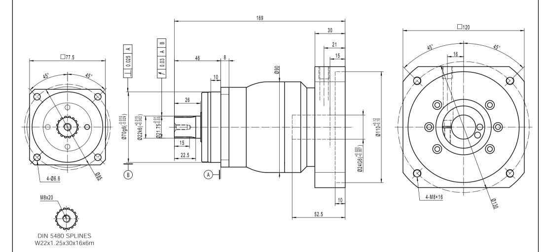
Note 1: This drawing shows the dimensions of X-Treme-SQ-ST-075 - 1 STAGE (this drawing is common to all ratios from 3 to 10)
