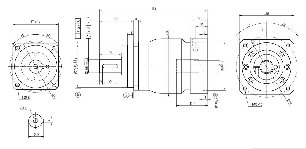
Note 1: This drawing shows the dimensions of X-Treme-SQ-ST-075 - 1 STAGE (this drawing is common to ratios 3 to 10)
