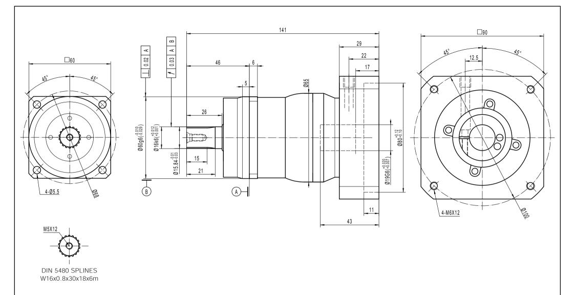
Note 1: This drawing shows the dimensions of X-Treme-SQ-ST-060 - 1 STAGE (this drawing is common to ratios 3 to 10)
