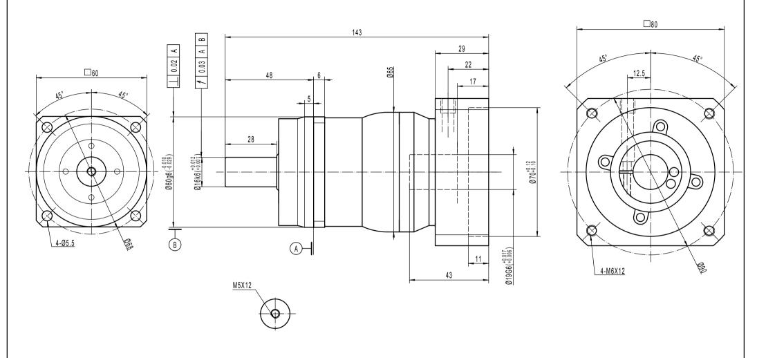
Note 1: This drawing shows the dimensions of X-Treme-SQ-ST-060 - 1 STAGE (this drawing is common to ratios 3 to 10)
