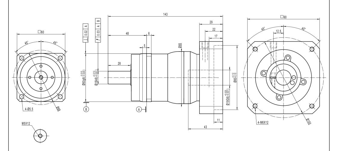
Note 1: This drawing shows the dimensions of X-Treme-SQ-ST-060 - 1 STAGE (this drawing is common to ratios 3 to 10)
