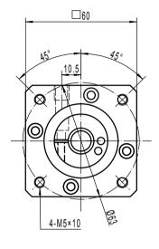
Note 1: This drawing shows the dimensions of WISER-SQ-ST-090 - 2 stages (It is common to all ratios from 12 to 100)
