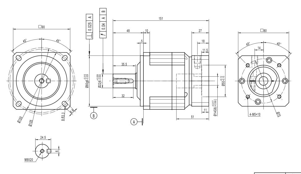
Note 1: This drawing shows the dimensions of Wiser-SQ-ST-090 - 1 STAGE (this drawing is common to ratios 3 to 10)
