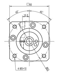
Note 1: This drawing shows the dimensions of Wiser-SQ-ST-060 - 1 STAGE (this drawing is common to ratios 3 to 10)
