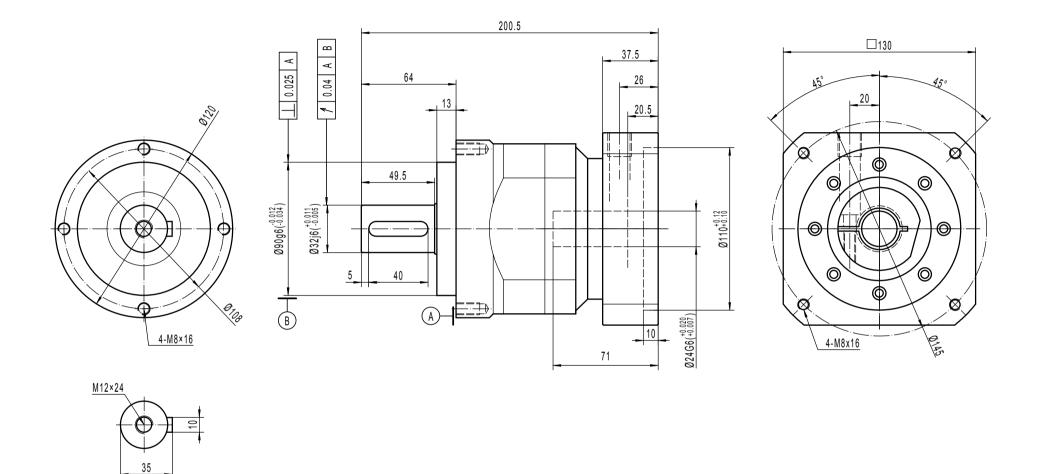
Note 1: This drawing shows the dimensions of WISER-CI-ST-120 - 1 STAGE (this drawing is common to ratios 3 to 10)
