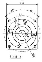
Note 1: This drawing shows the dimensions of WISER-CI-ST-090 - 2 stages (It is common to all ratios from 12 to 100)
