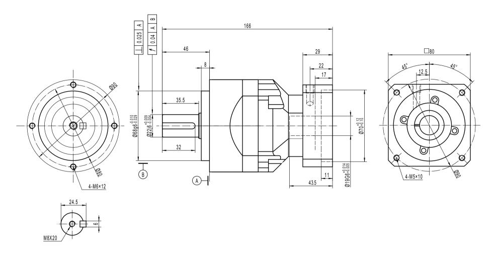
Note 1: This drawing shows the dimensions of WISER-CI-ST-090 - 2 stages (It is common to all ratios from 12 to 100)
