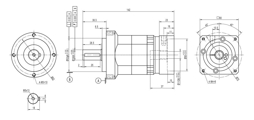
Note 1: This drawing shows the dimensions of WISER-CI-ST-060 - 2 stages (It is common to all ratios from 12 to 100)
