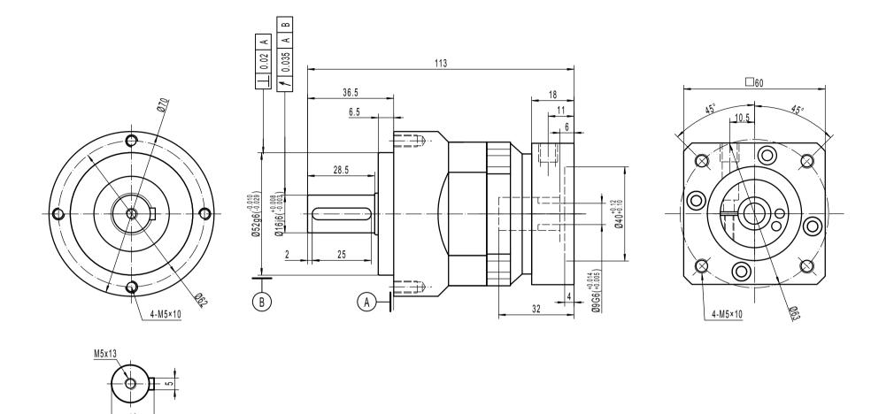
Note 1: This drawing shows the dimensions of Wiser-CI-ST-060 - 1 STAGE (this drawing is common to ratios 3 to 10)
