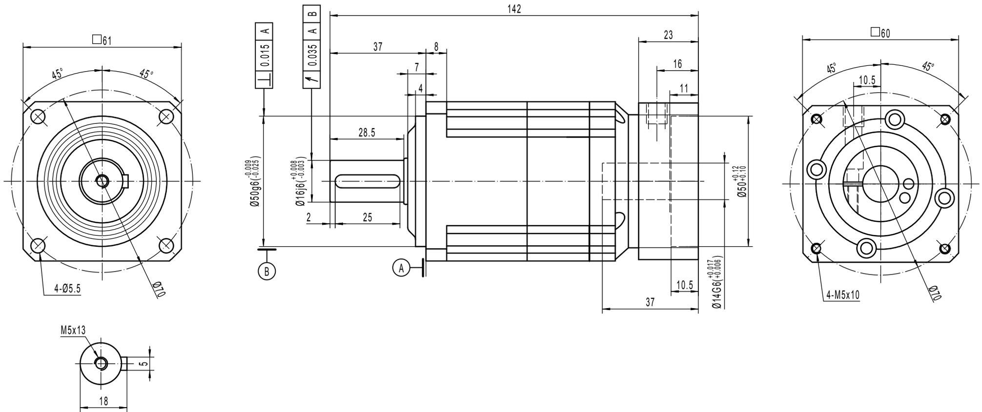
Note 1: This drawing shows the dimensions of WISER-SQ-ST-060 - 2 STAGES (this drawing is common to ratios 12 to 100)
