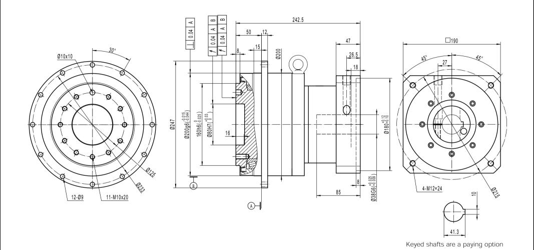
Note 1: This drawing shows the dimensions of ULTIMATE-CI-ST-200 - 2 STAGES (this drawing is common to all ratios from 16 to 100)
