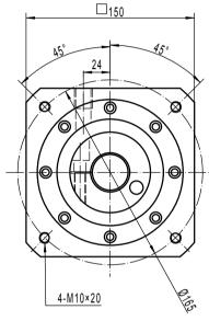
Note 1: This drawing shows the dimensions of ULTIMATE - CI - ST - 200 - 2 STAGES (this drawing is common to all ratios from 16 to 100)
