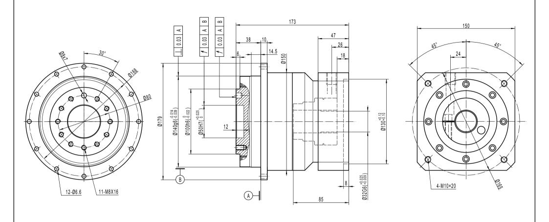
Note 1: This drawing shows the dimensions of ULTIMATE-CI-ST-140 - 1 STAGE (this drawing is common to all ratios from 4 to 10)
