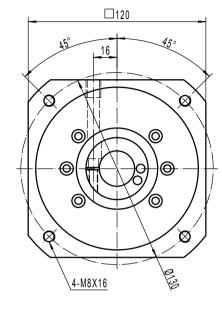
Note 1: This drawing shows the dimensions of ULTIMATE - CI - ST - 110 - 2 STAGES (this drawing is common to ratios 16 to 100)
