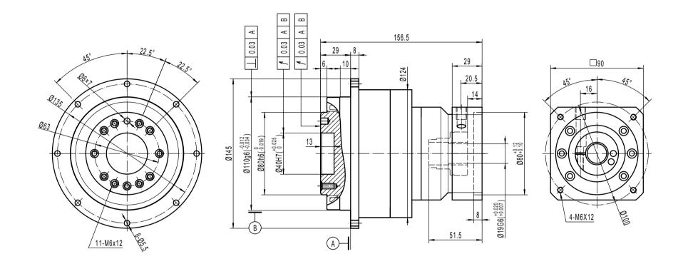
Note 1: This drawing shows the dimensions of ULTIMATE - CI - ST - 110 - 2 STAGES (this drawing is common to all ratios from 16 to 100)
