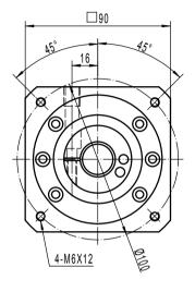
Note 1: This drawing shows the dimensions of Ultimate – CI – ST – 110 2 STAGES (this drawing is common to ratios 16 to 100)
