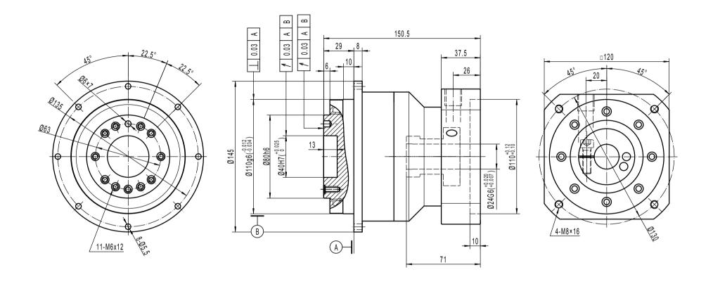
Note 1: This drawing shows the dimensions of ULTIMATE-CI-ST-110 - 1 STAGE (this drawing is common to all ratios from 4 to 10)
