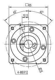
Note 1: This drawing shows the dimensions of ULTIMATE - CI - ST - 090 - 2 STAGES (this drawing is common to ratios 16 to 100)
