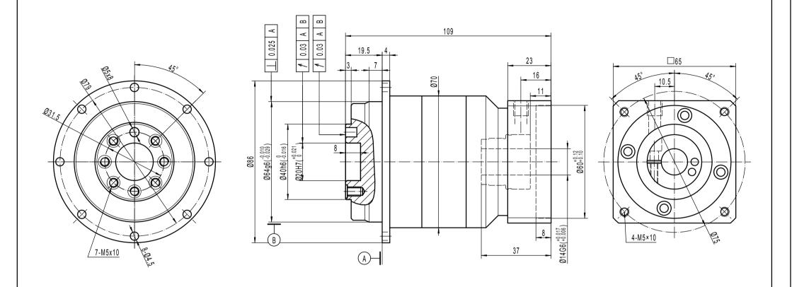
Note 1: This drawing shows the dimensions of ULTIMATE-CI-ST-064 - 2 STAGES (this drawing is common to all ratios from 16 to 100)
