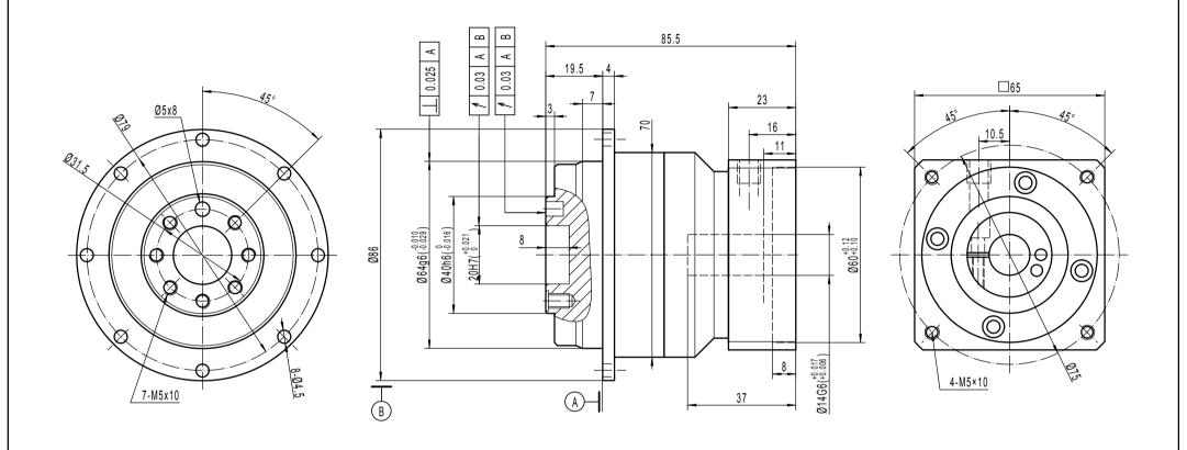
Note 1: This drawing shows the dimensions of ULTIMATE – CI – ST – 064 – 1 STAGE (this drawing is common to all ratios from 4 to 10) Note 2: Full technical ratings can be found on www.reckondrives.com
