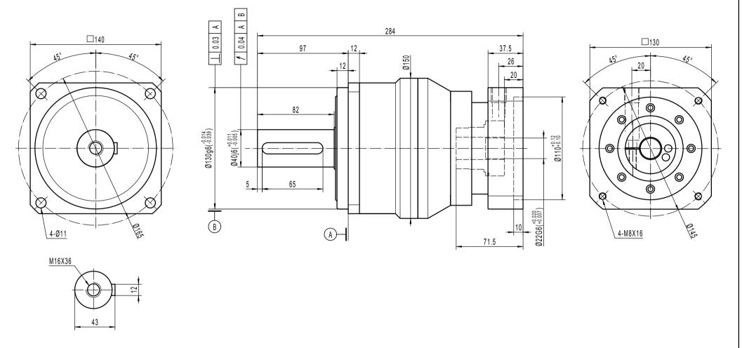
Note 1: This drawing shows the dimensions of LIVELY-SQ-ST-140 - 2 stages (It is common to all ratios from 12 to 100)
