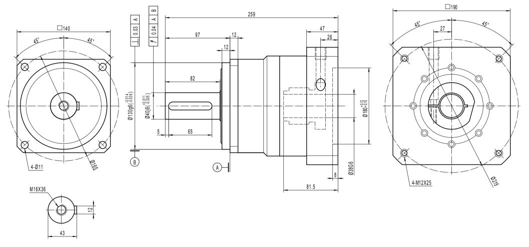
Note 1: This drawing shows the dimensions of Lively-SQ-ST-140 - 1 STAGE (this drawing is common to ratios 3 to 10)
