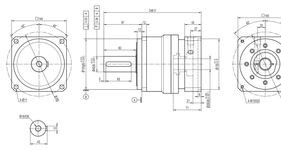
Note 1: This drawing shows the dimensions of Lively-SQ-ST-140 - 1 STAGE (this drawing is common to ratios 3 to 10)
