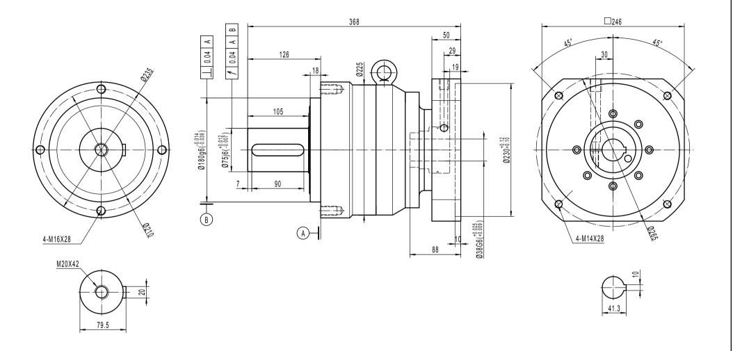
Note 1: This drawing shows the dimensions of Lively – CI – ST – 235 – 2 stages (It is common to all ratios from 12 to 100)
