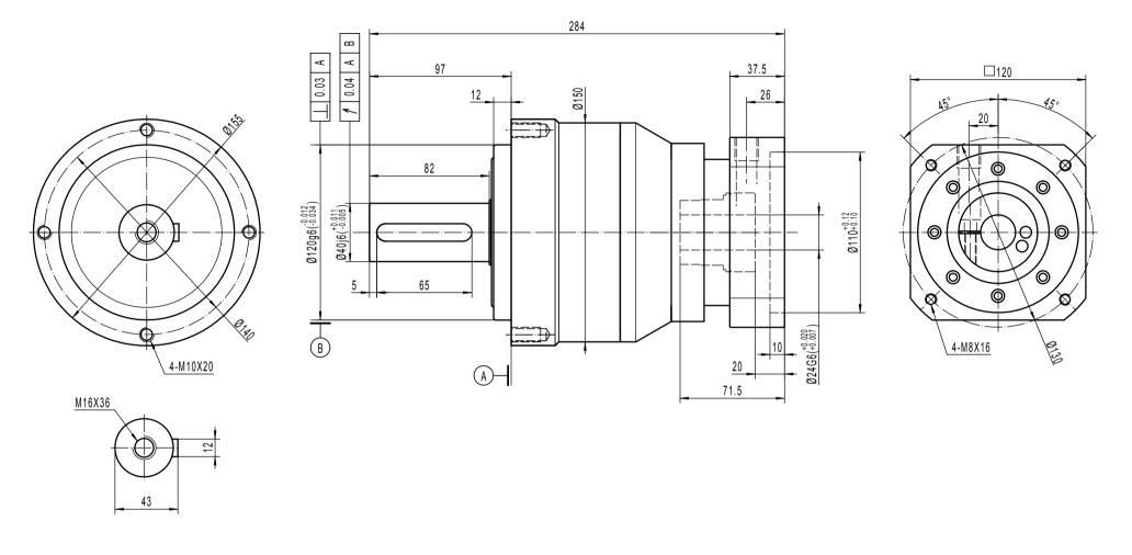
Note 1: This drawing shows the dimensions of LIVELY-CI-ST-155 - 2 STAGES (this drawing is common to ratios 12 to 100)
