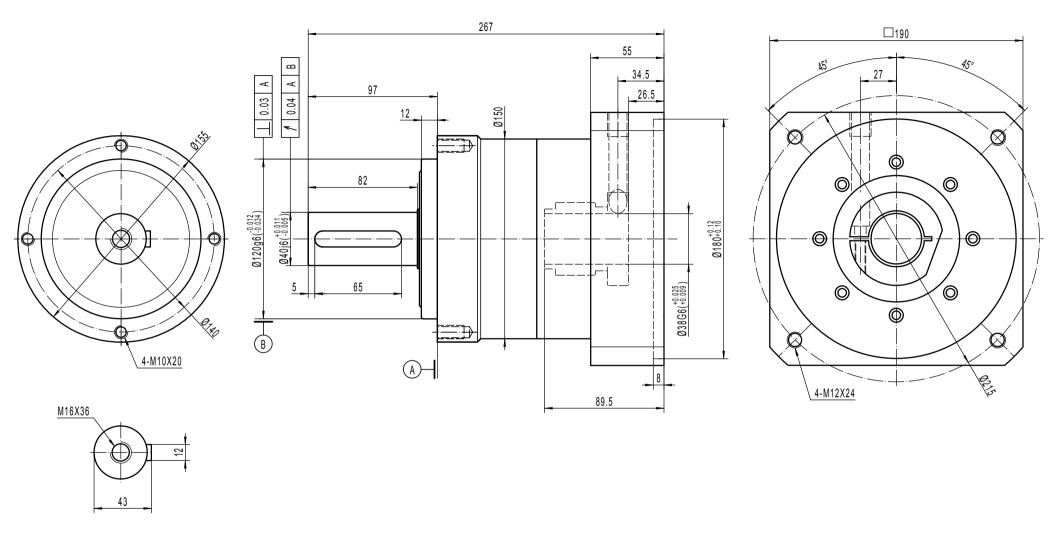
Note 1: This drawing shows the dimensions of Lively-CI-ST- 155- 1 STAGE (this drawing is common to ratios 3 to 10)
