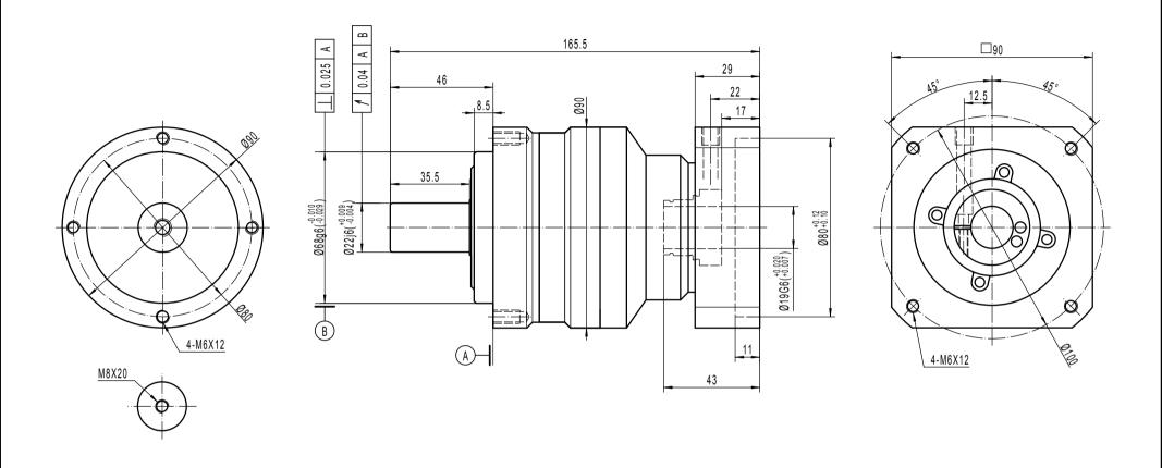
Note 1: This drawing shows the dimensions of LIVELY-CI-ST-090 - 2 stages (It is common to all ratios from 12 to 100)
