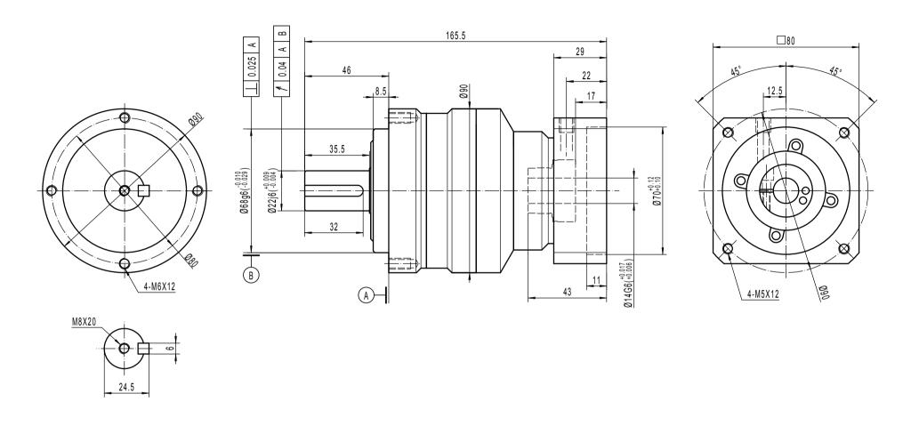
Note 1: This drawing shows the dimensions of Lively-CI-ST-090 - 2 stages (It is common to all ratios from 12 to 100)
