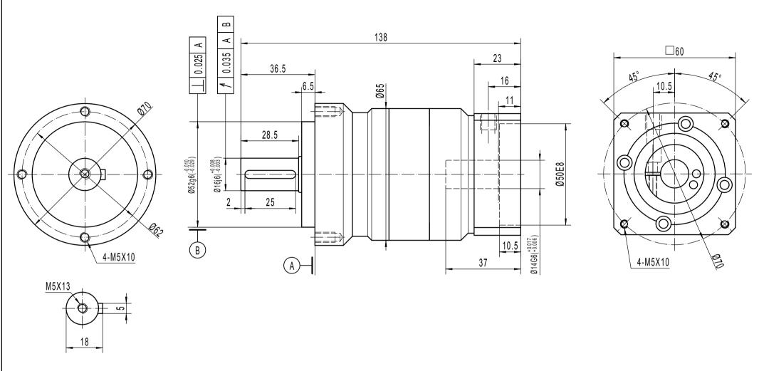
Note 1: This drawing shows the dimensions of Lively-CI-ST-060 - 2 stages (It is common to all ratios from 12 to 100)
