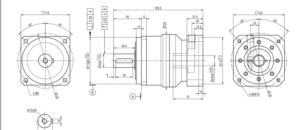
Note 1: This drawing shows the dimensions of BOOSTER-SQ-ST-120 - 1 STAGE (this drawing is common to ratios 3 to 10)
