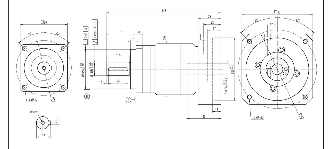
Note 1: This drawing shows the dimensions of BOOSTER-SQ-ST-060 - 2 stages which are common to all ratios from 12 to 100)
