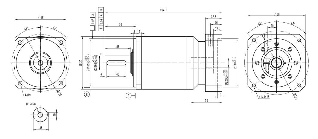
Note 1: This drawing shows the dimensions of ACCESS-SQ-ST-120 - 2 stages (It is common to all ratios from 12 to 100)
