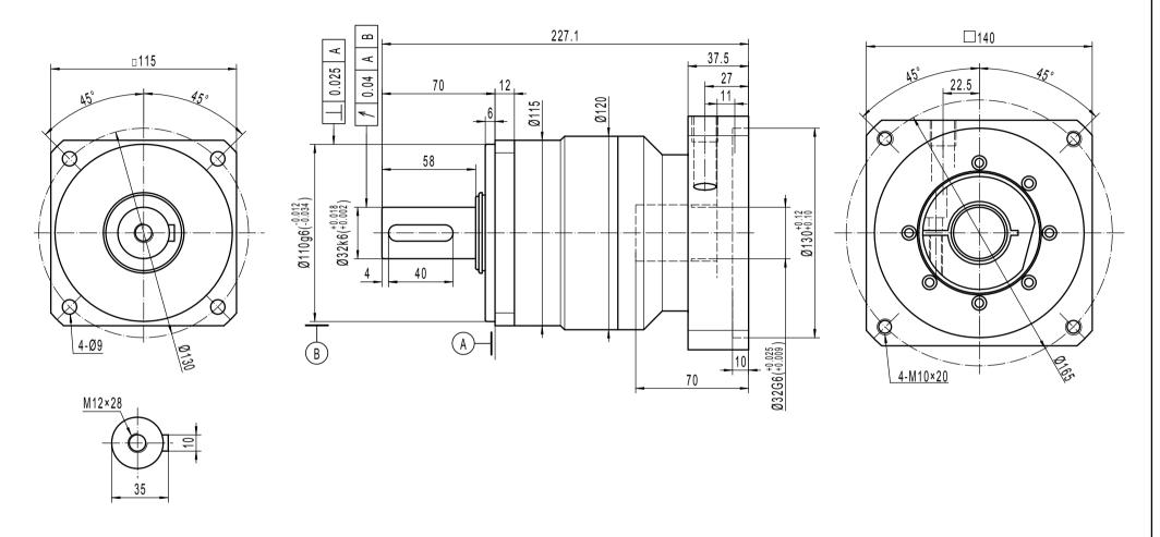
Note 1: This drawing shows the dimensions of ACCESS-SQ-ST-120 - 1 STAGE (this drawing is common to ratios 3 to 10)
