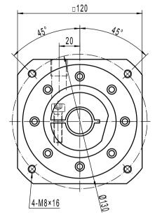
Note 1: This drawing shows the dimensions of ACCESS-SQ-ST-120 - 1 STAGE (this drawing is common to ratios 3 to 10)
